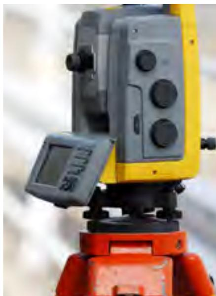
Surveyors use the Total Station Theodolite to measure distances and angles.
